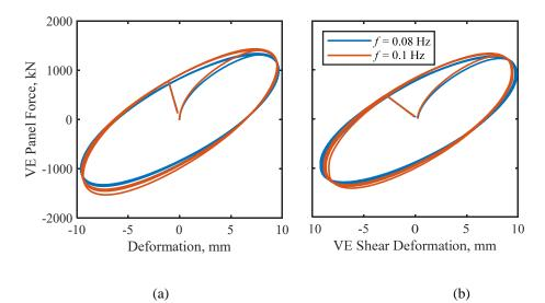
Figure 9. (a) Harmonic hysteresis from MTS test at at  $\gamma = 100\%$  and comparison (b) with Full scale shear set up.
