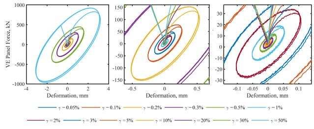
Figure 6. VE Panels A hysteretic response from small to large strains at f = 0.3 Hz.
