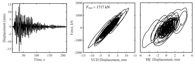
Figure 10. (a) Service level earthquake testing Protocol (b) VCD hysteresis (c) VE damper panel hysteresis
