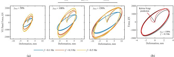
Figure 5. (a) VE Panels A hysteretic response at various frequencies and strain amplitudes (b) Harmonic tests results at  $\gamma = 150\%$  and f = 0.3 Hz and comparison with Kelvin-Voigt model.
