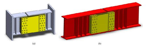
Figure 8. Full-scale outrigger VCD specimens (a) replaceable end plate VCD-R (b) concrete wall embedded VCD-E
