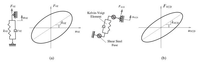
Figure 3. (a) Kelvin Voigt model for VE materials and hysteretic response, (b) Viscoelastic-plastic VCD model and viscoelastic hysteretic response
