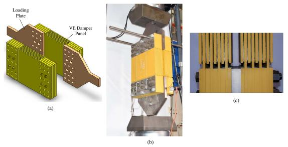
Figure 4. (a) VE panels testing assembly, (b) MTS experimental setup, (c) VE panels deformation for  $\gamma = 150\%$ .
