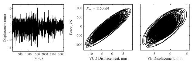
Figure 11. (a) Design level wind testing Protocol (b) VCD hysteresis (c) VE damper panel hysteresis
