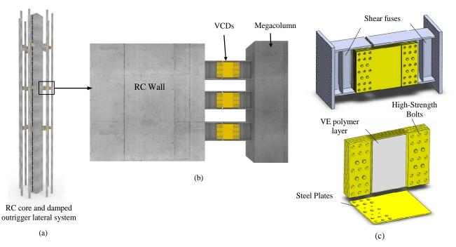
Figure 1. (a) Damped VCD high-rise building, (b) Outrigger detail, (c) VCD and VE panel
